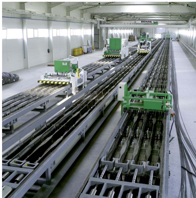
Figure 1 Typical view from inside a sleeper plant using the production method of Abetong
