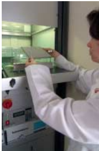
3 Measuring apparatus for determination of NO x degradation rates in the laboratory
